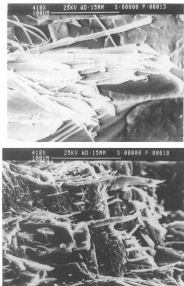
Figure 8 Scanning electron micrographs of fracture surfaces of uncompatibilized PP/Vectra B 2/8 (top) and compatibilized PP/Vectra B 2/8 (bottom) plaques. Fracture is along the flow direction
