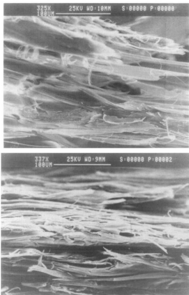
Figure 6 Scanning electron micrographs of fracture surfaces of uncompatibilized PP/Vectra B 8/2 (top) and compatibilized PP/Vectra B 8/2 (bottom) plaques. Fracture is along the flow direction
