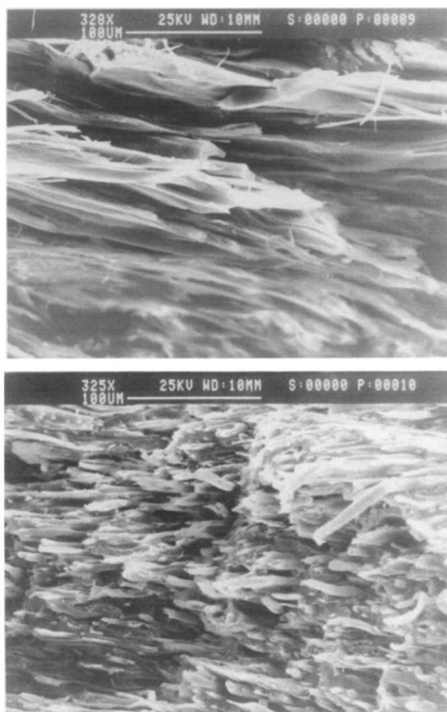
Figure 7 Scanning electron micrographs of fracture surfaces of uncompatibilized PP/Vectra B 5/5 (top) and compatibilized PP/Vectra B 5/5 (bottom) plaques. Fracture is along the flow direction
